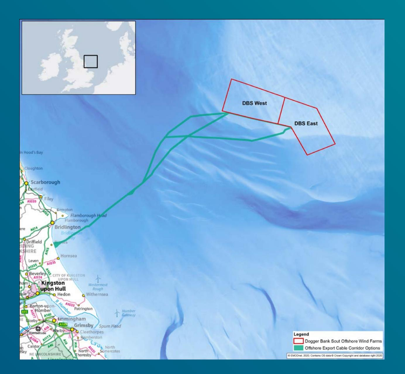
The offshore export cables would make landfall near Skipsea, where they would be connected to the onshore cables in transition joint bays (TJB), having been installed under the intertidal zone by HDD. More information on the TJBs can be found on the landfall information banner.
